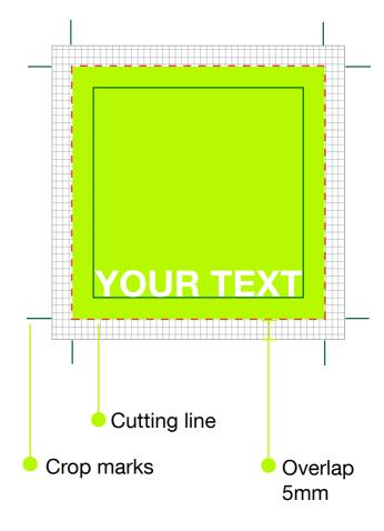
The overlap must be at least 5 mm above the cutting contour.
